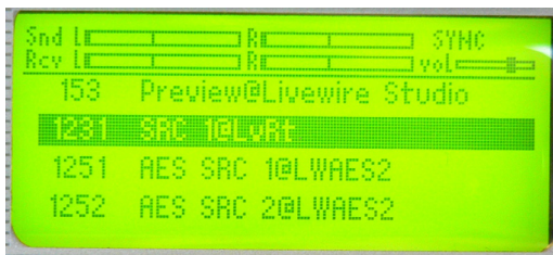
Figure 2-3: Router Selector - Source Selection
