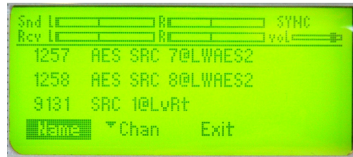
Figure 2-3: Router Selector - Source List
